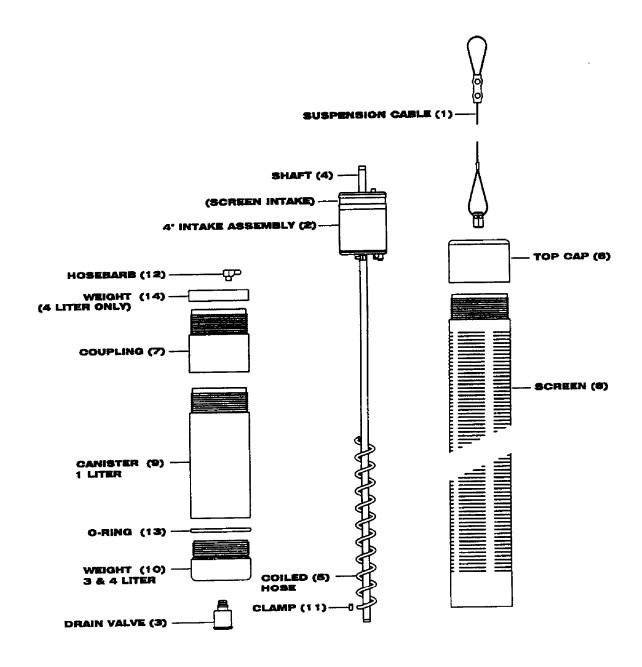
Figure 6 – Standard 4" PRC Skimmer Assembly (3&4 Liter) Parts List 16
