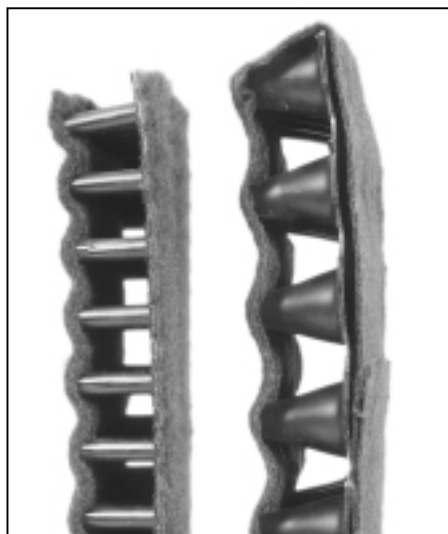
Figure 2. Typical open core geocomposite panel drains: post & net (left), cusped (right)
